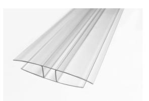
Marlon ST H-profiles are designed to cover the joints between multiwall sheets. They are not structural and should be fully supported along their entire length. They should not be considered weather-tight which limits their use to horticulture, agriculture and simple canopies. The profile should be secured to the sub structure at approximately 500mm centres.
